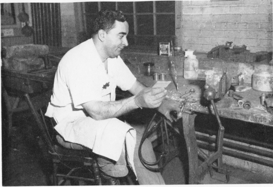
Salvatore Tolla, Solder Room brazer, is preparing a carboly tool bit to be placed by "brazing" on a machine tool shank. This is one of the most important jobs done by Salvatore. The attachment of these modern tool bits to the shanks is a great aid to high speed war production.
